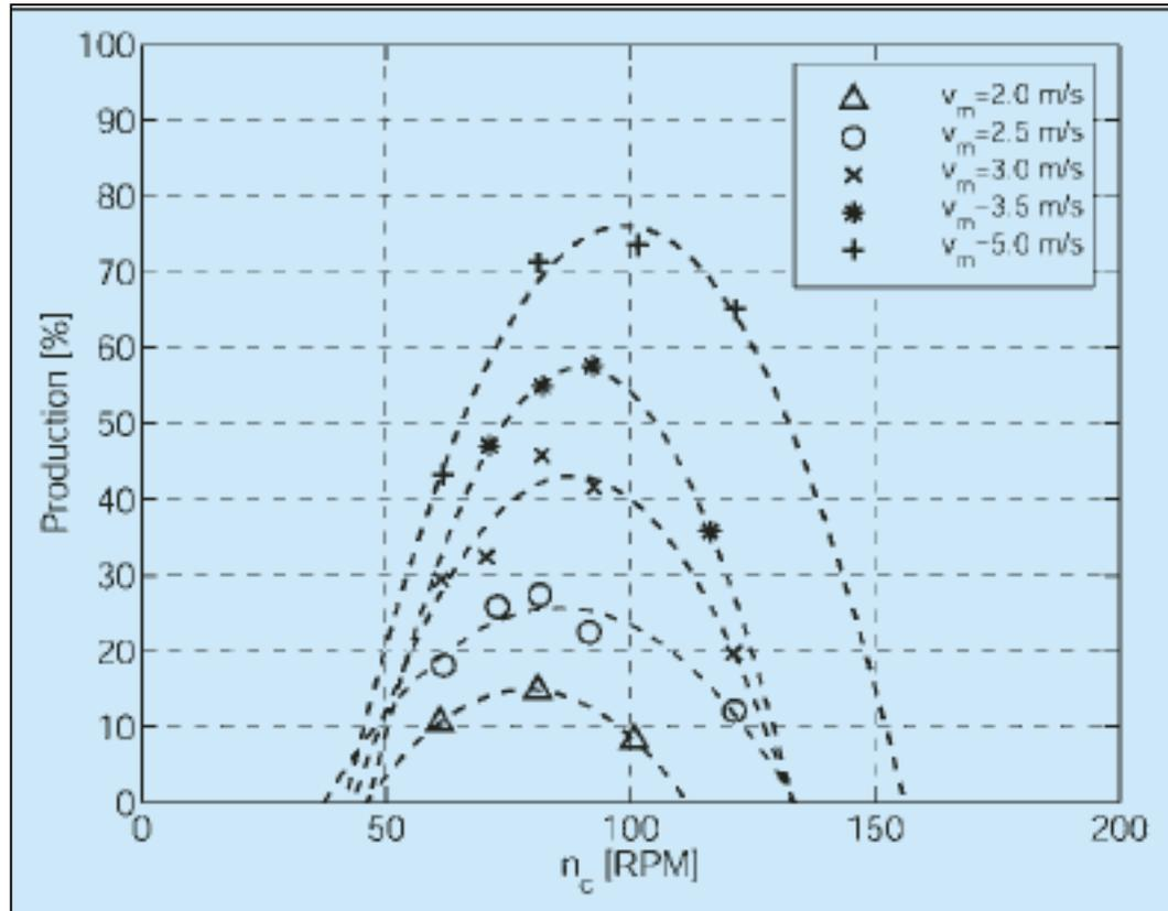
Production versus RPM of cutter head for different mixing suction velocities
