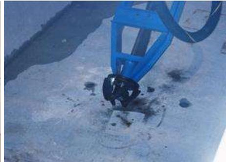
Rotary Cutter Head Setup in Tank
