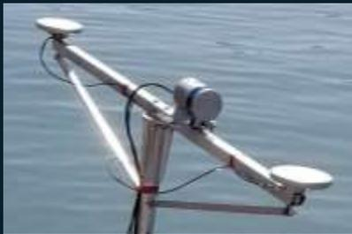
Dual head NORBIT **STX** with integrated **Lidar** and **GNSS/INS**
