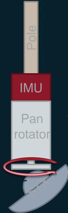
Coarse rotation synced to rock depositing arm direction to keep STX scanning on a rea
