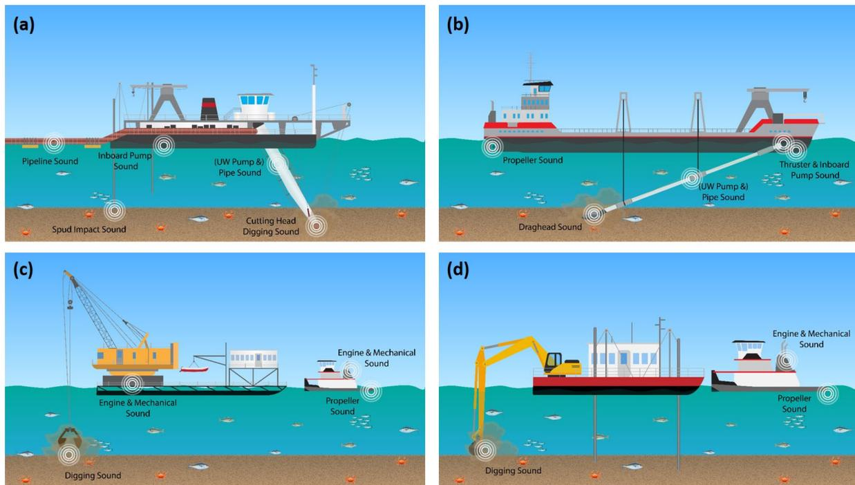
**Figure 1. Examples of hydraulic (top) and mechanical (bottom) dredge types and potential sound sources (adapted from CEDA 2011). (a) cutter suction dredge (CSD); (b) trailing suction hopper dredge (TSHD); (c) grab dredge (GD); and (d) backhoe dredge (BHD)**
