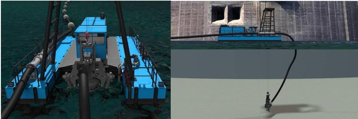
Illustration of the dredging system based on submersible pumps developed for deep-water applications
