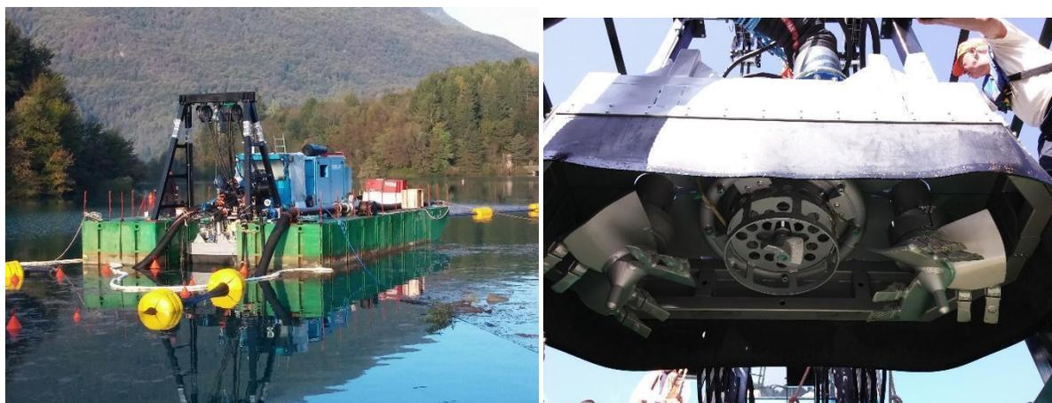
Dredging system used at Ambiesta Reservoir; photographs of the complete dredge and submersible dredging pump anti-turbidity shroud
