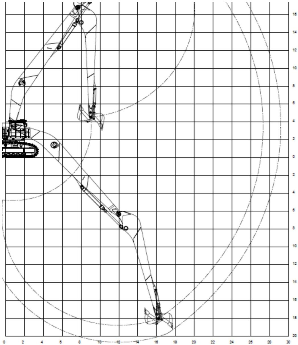
Figure 1. Concept of working range diagram for modified hydraulic excavator.
