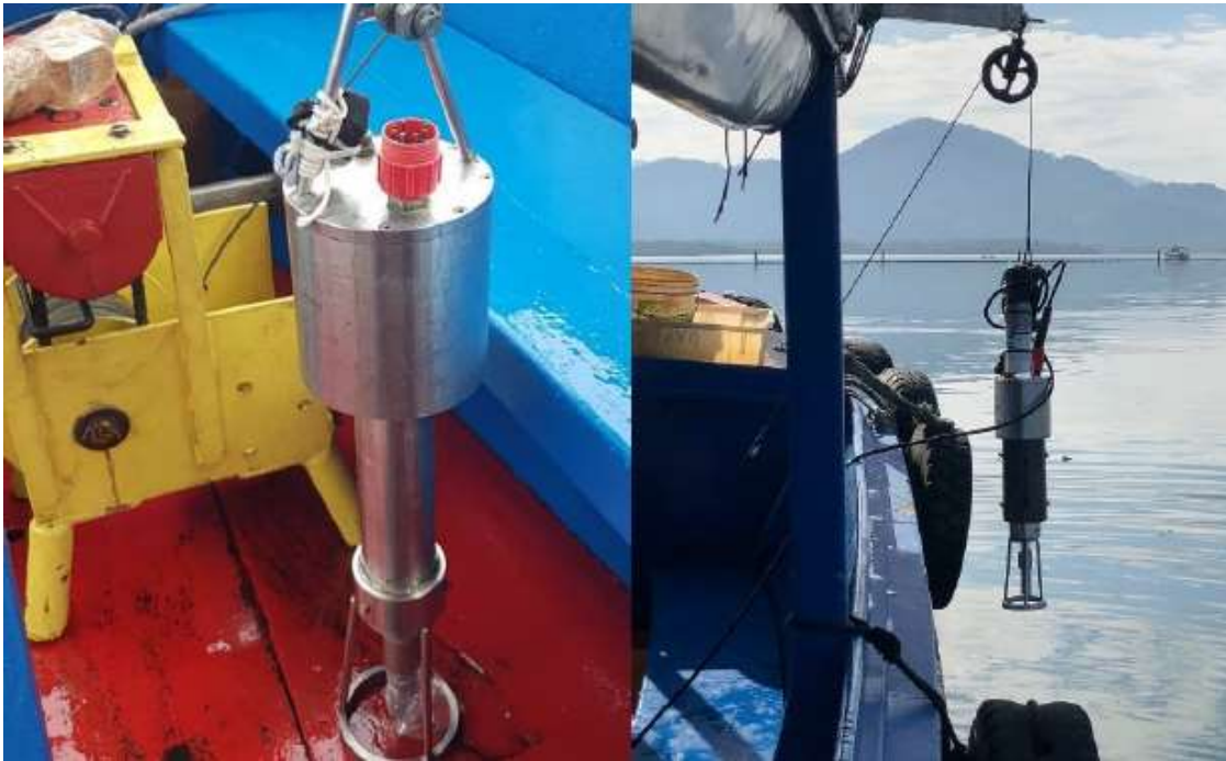
Figure 11. Inside CAD material density survey monitoring using DensiTune equipment.
