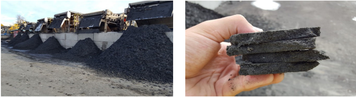
Figure 6. Filter cake from belt filter presses used in Phase II.
