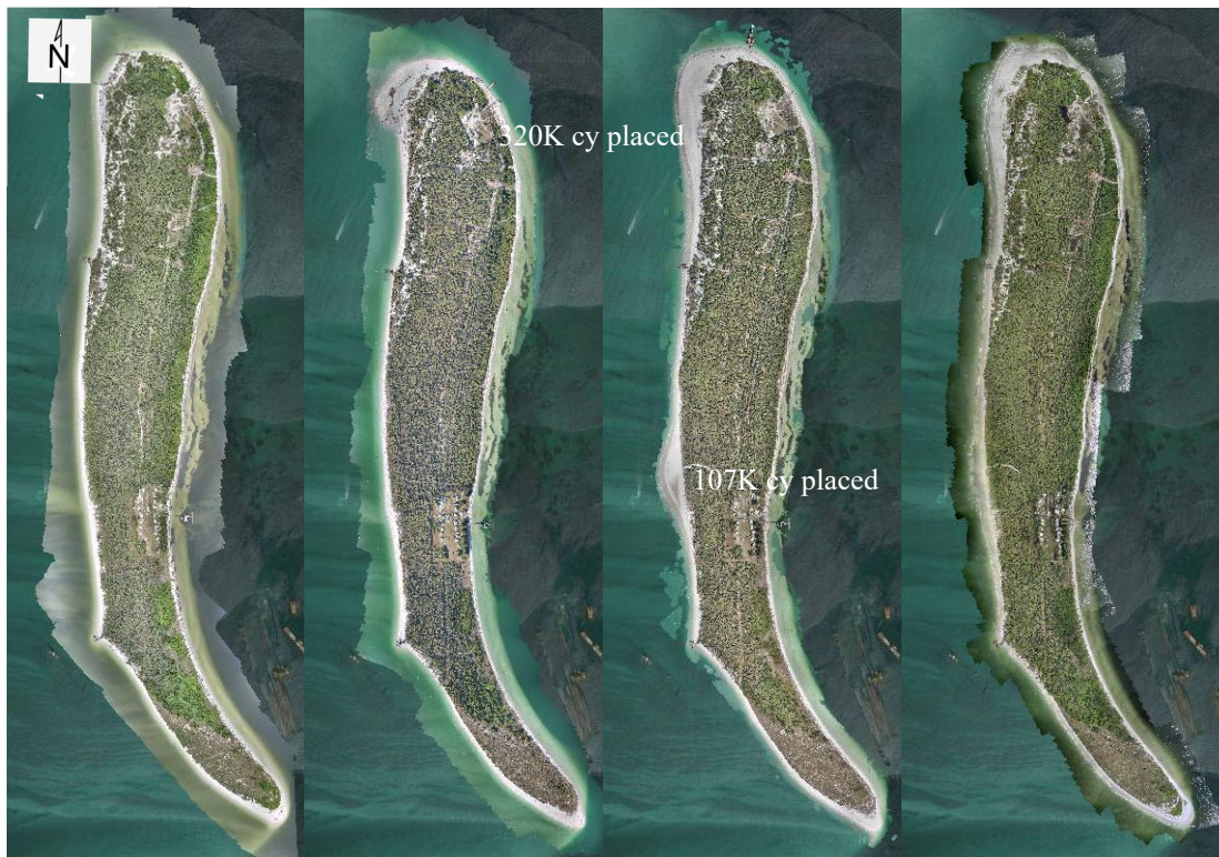
Figure 16. UAV aerial mosaics (left to right) pre-placement 6 October 2014, during placement 16 December 2015, ten days post-placement 16 March 2015, five months post-placement 17 August 2015.
