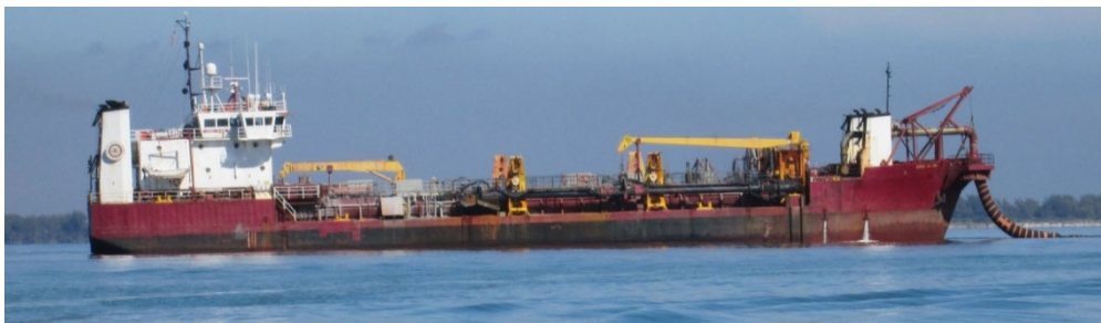
Figure 3. The Dodge Island, a GLDD hopper dredge, pumping out material to Egmont Key, FL on 16 December 2014.
