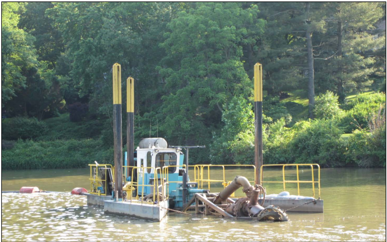
JND Thomas's 8-Inch DSC Dredge at Wilde Lake in Columbia, Maryland (Photo Courtesy of Columbia Association)
