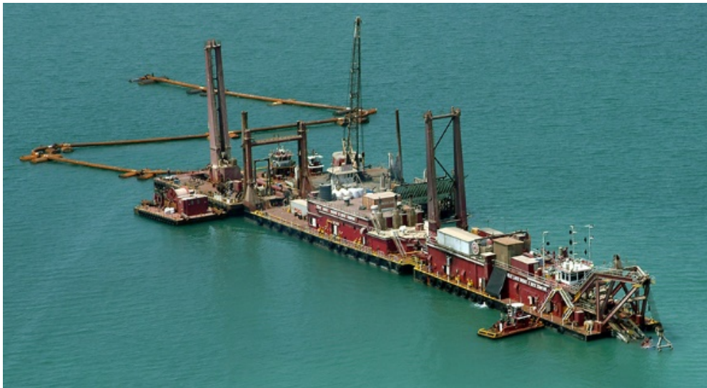
Figure 1. Cutter suction dredge “California” showing spud carriage and pipeline (Courtesy of Great Lakes Dredge and Dock).
