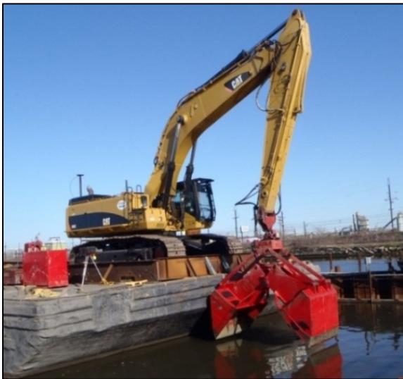
Figure 6. Level-cut clamshell dredge
