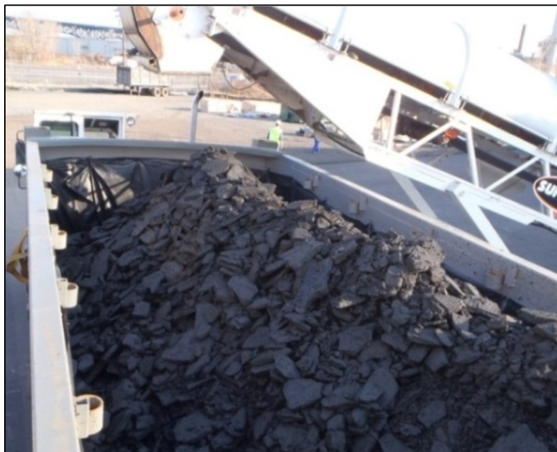
Figure 14. Filter cake loaded into intermodal container
