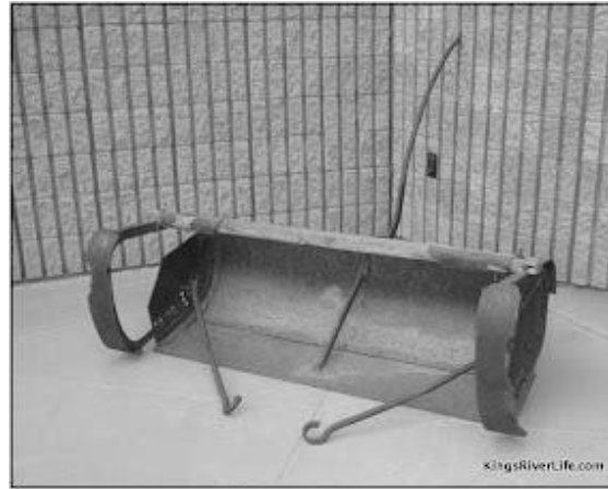
Fresno Scrapper, invented by James Porteous, 1883
