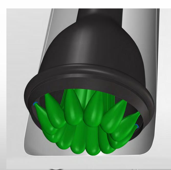
The recycled water is injected through an air injection nozzle into the base of the suction pipe.
