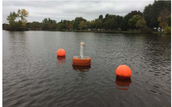
Photo 2: Solar powered remote monitoring buoy
