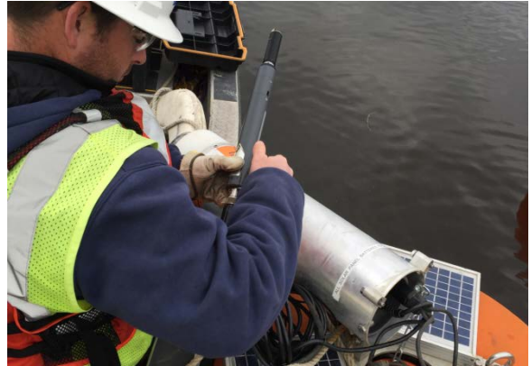
Photo 8: Calibrating turbidity buoy
