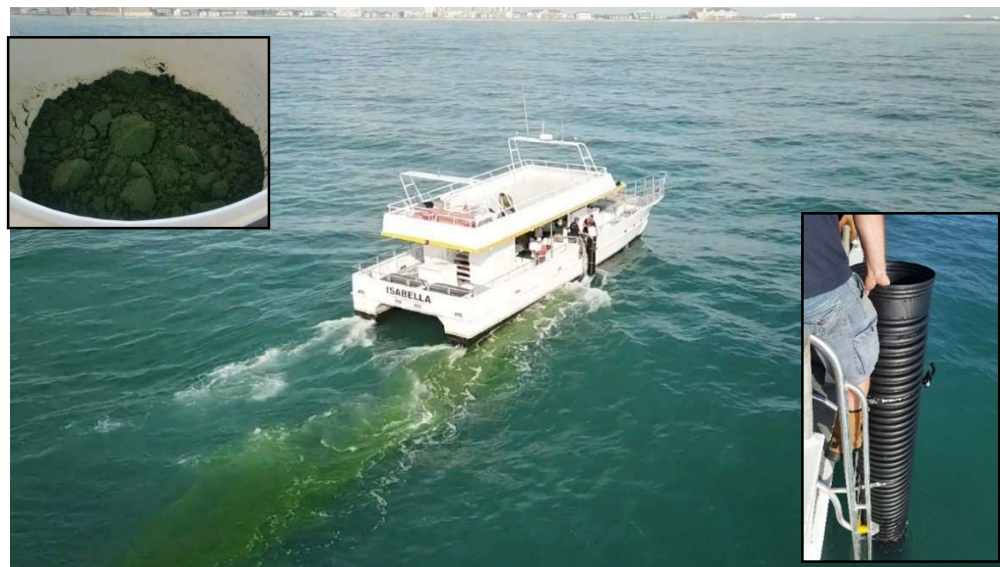
Figure 2. Photo of tracer deployment. 2000 kg (4,400 lb) of ferrimagnetic fluorescent tracer particles (top left inset) engineered to match the hydraulic characteristics of the dredged material were released via a chute on the side of the boat (bottom right inset) over the top of the nearshore berm in August 2018 (Inset photograph in the upper left courtesy of Partrac GeoMarine Inc.; large photograph and inset photograph in the lower right courtesy of the City of South Padre Island).
