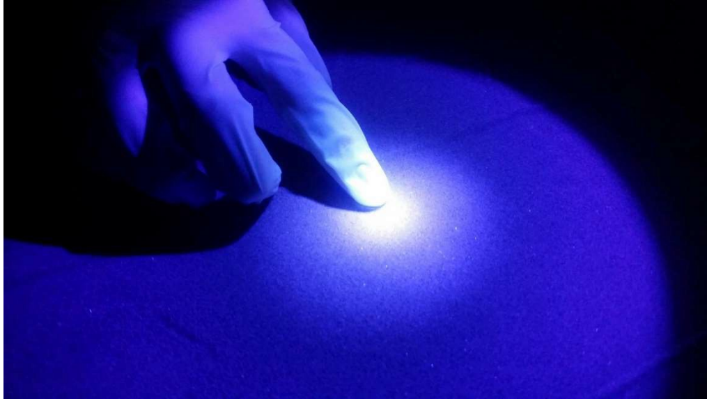
Figure 4. Photo of laboratory tracer assessment. Surface grab samples were dried and spread out on a flat PVC tray. A 12,000-Gauss cylindrical magnet was used to extract the ferrimagnetic fluorescent tracer particles for subsequent counting under blue light illumination.
