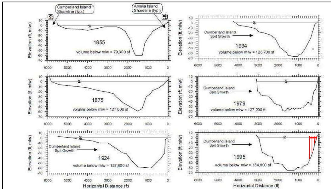
Figure 10 – Controlling bathymetric cross-sections at the throat of St. Mary's Entrance between Fort Clinch and Cumberland Island. Historical shoreline positions are also depicted in order to illustrate the relationship between the growth of the Cumberland Island spit and southerly channel migration. (From Raichle *et al.* 1995)
