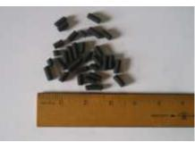
Carbon %: 40% w/w Typical Size: 1/4" Minus Diam. Length Varies (6.7 mm diam.) Bulk Density: 45lb/cu.ft.
