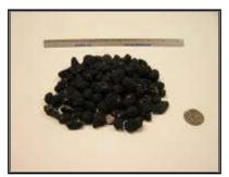
Carbon %: 10% w/w Typical Size: 3/8" Minus (9.5 mm) Bulk Density: 65-75/cu.ft.
