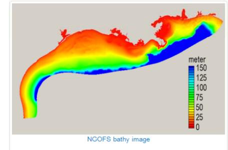
The NGOFS grid has 91,652 nodes and 17,6545 elements. Grid resolution ranges from 10 km on the open ocean boundary to approximately 600 m near the coast, indicating the flexibility of the grid size based on bathymetry from the deep ocean to the coast.
