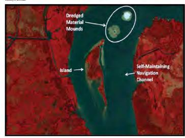
Figure 1: December 2011 aerial infrared photograph of the Atchafalaya River island after multiple years of upstream mounting of dredged material. The island's formation has reduced the overall cross sectional area of the river, increasing river flow through the maxingtion channel to the east sufficient to reduce shoaling and maintenance dredsing reastivements.
