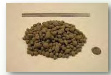
**Aggregate:** Nominal AASHTO #8 (1/4-3/8") or custom-sized to meet project-specific need \* Limestone or non-calcareous substitute, as deemed project-appropriate
