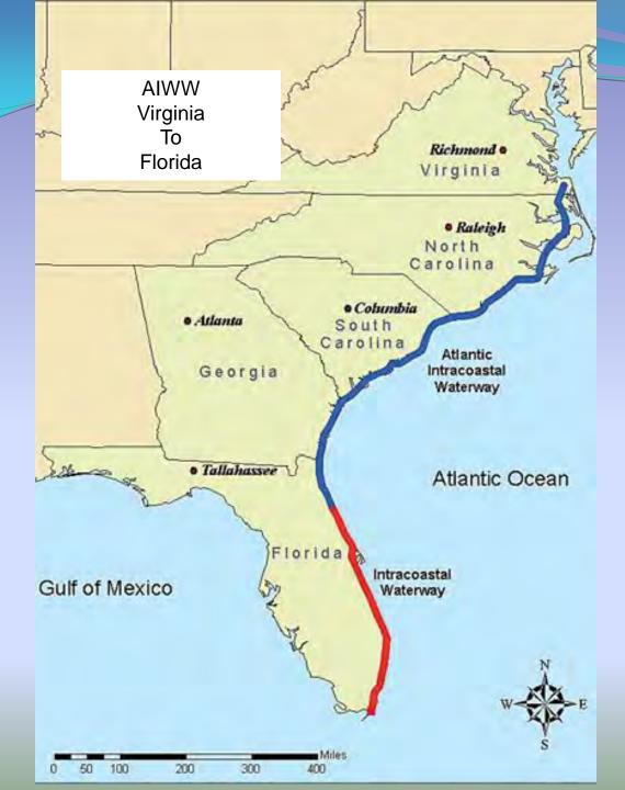
**The US Army Corps of Engineers** maintains the Waterway for 1,100 miles between Norfolk, Virginia and Florida Bay, Florida. M-95 is authorized to -12 feet MLLW with widths of 90 feet through land cuts and 150 feet in open water areas, and -10 feet MLLW in most of Florida.
