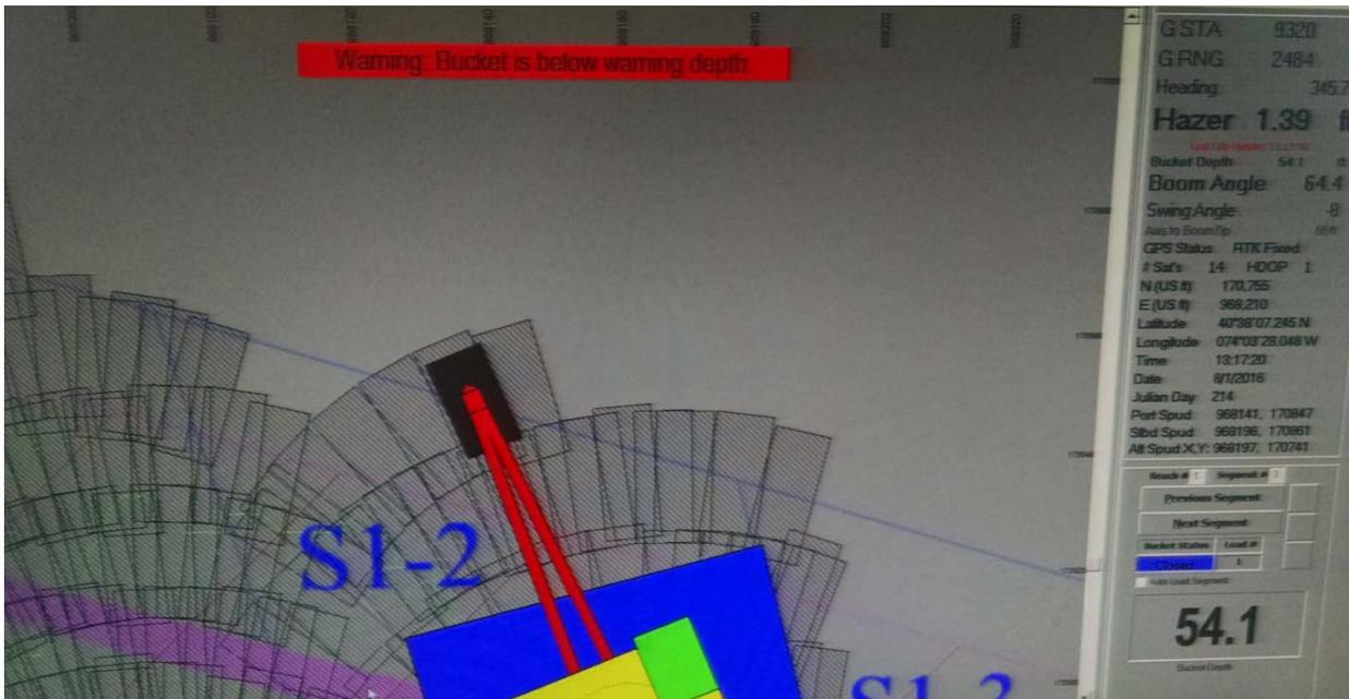
Figure 6. Screen Shot of Contractor's Dredge Control Software
