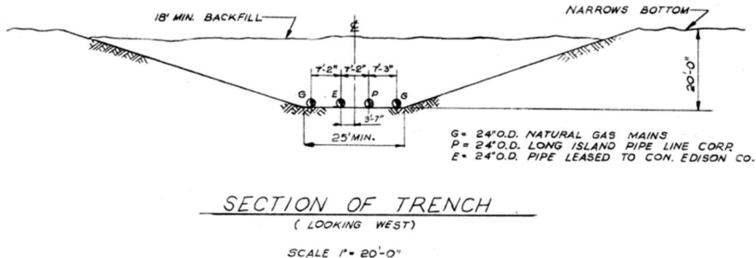
Figure 2. Typical Cross-section of Utilities (looking West)
