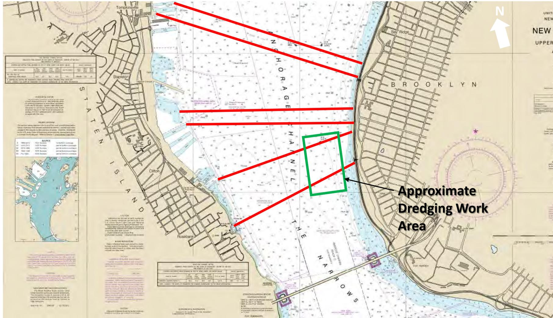
Figure 1. Some of the Designated Utility Crossings (red lines) at New York Harbor Navigation Channel
