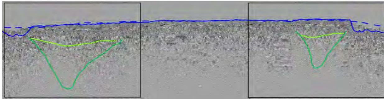
Figure 3. Sub-bottom profile imagery Indicating Utility Trench Location (looking East/West)
