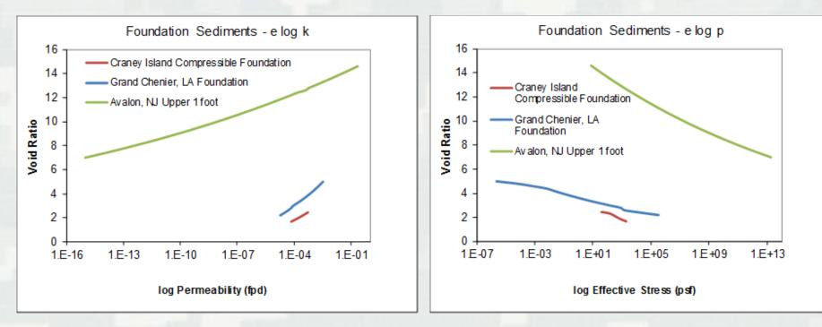
Foundation sediment was not sampled. Used several surrogate consolidation curves to evaluate potential compression of the foundation material.
