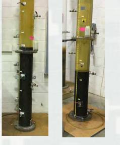
Kettle Creek and Good Luck Point – completed column settling tests
