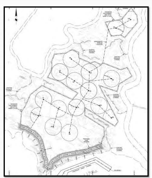
As-Built Pipe and Valve Network
