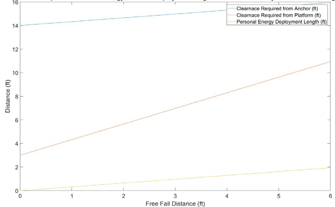
Required Clearance for a 220 lb (100 kg) worker using a 6 ft (1.8 m) lanyard for a free fall up to 6 ft (1.8 m)
