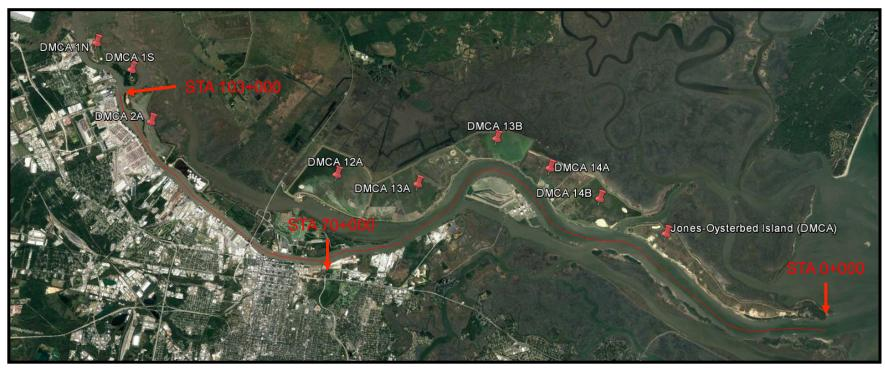
Requirement: Deepen the Inner Harbor from -42' MLLW to -47' MLLW; removing approximately 12 million cubic yards of new work material with disposal in DMCAs. Two contracts to be utilized for completion of deepening of the Inner Harbor for SHEP.
