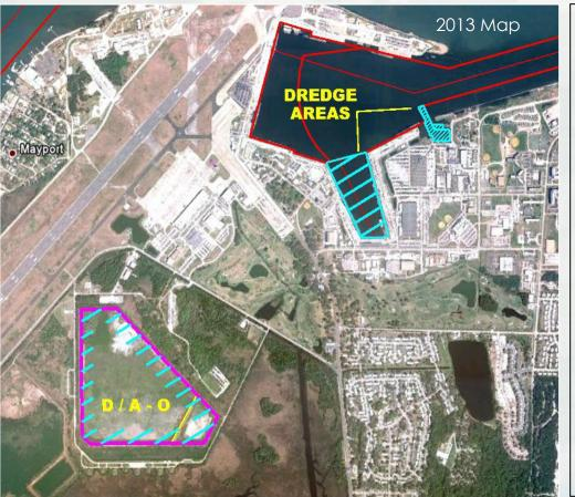
LOCATION: Duval County, Florida DREDGE TYPE: Hopper/Pipeline/Mechanical PLACEMENT: ODMDS QUANTITY: 1,400,000 CY DEPTH: 42 - 50 feet
