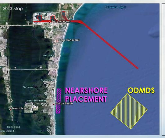
LOCATION: Brevard County, Florida DREDGE TYPE: Mechanical PLACEMENT: ODMDS & Nearshore QUANTITY: 2,000,000 CY DEPTH: 39 - 46 feet + 2 feet allowable overdepth
