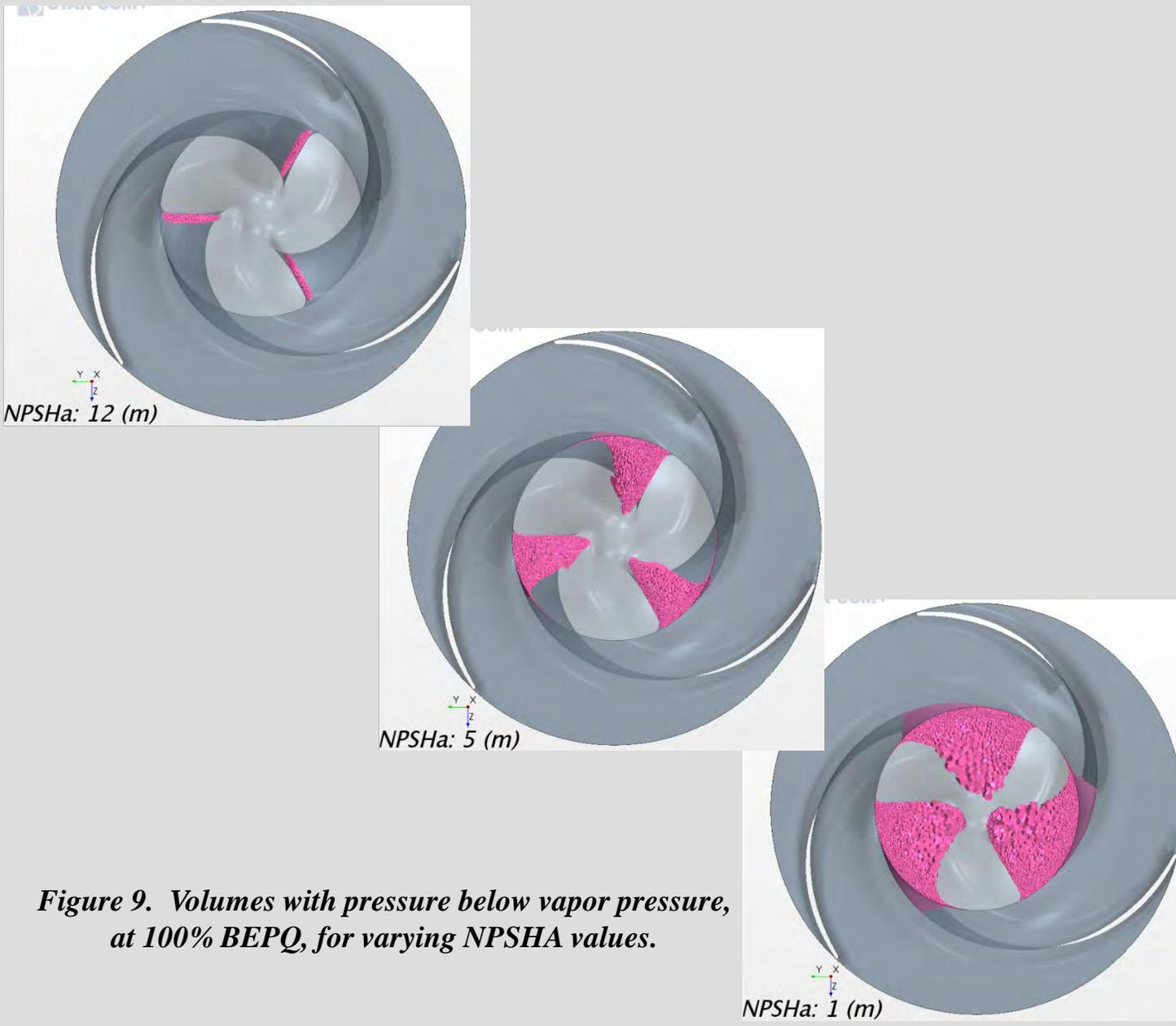
**Figure 9. Volumes with pressure below vapor pressure, at 100% BEPQ, for varying NPSHA values.**
