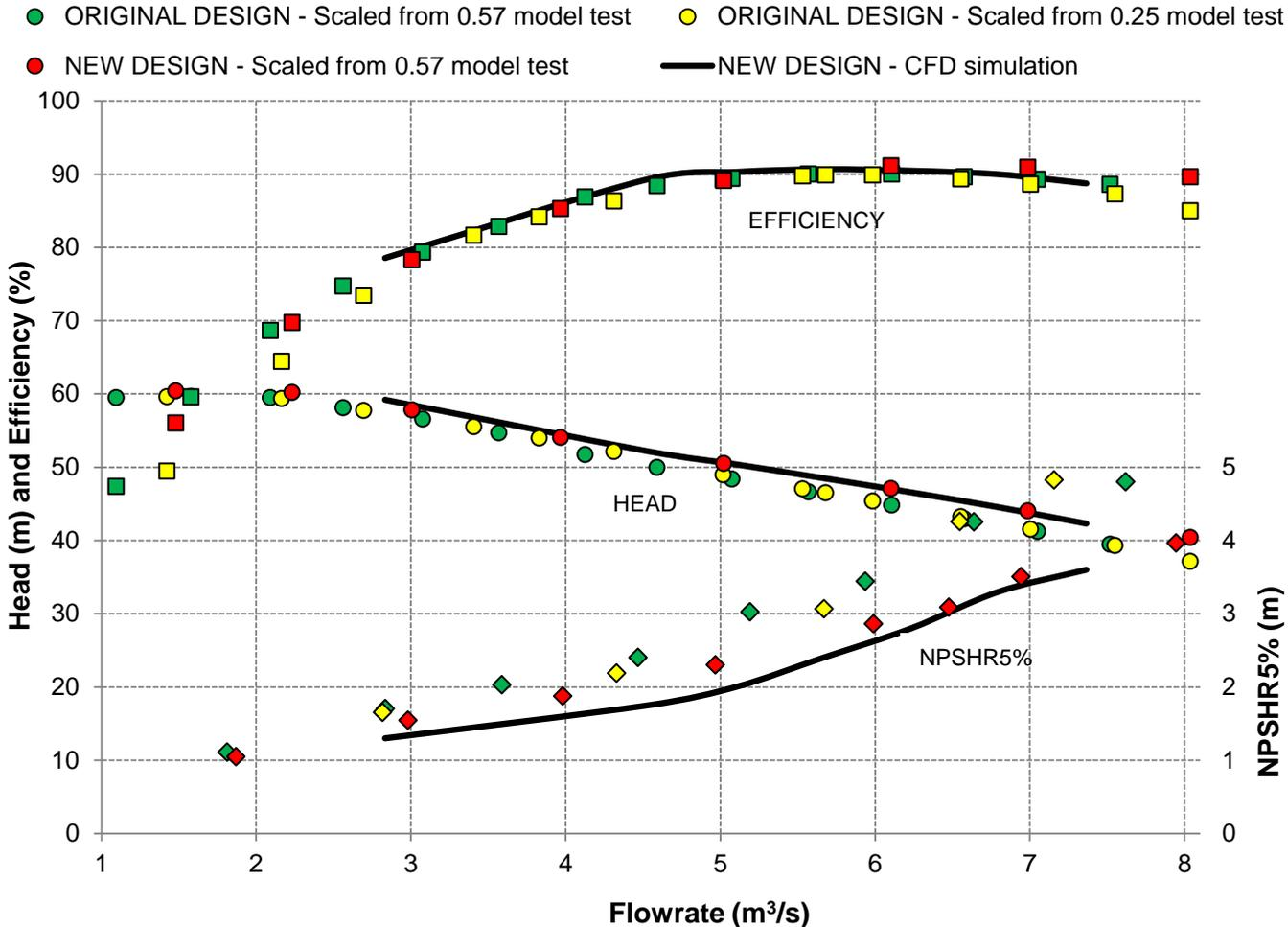
Figure 20 . Comparison of the three model pump tests and final design CFD.
