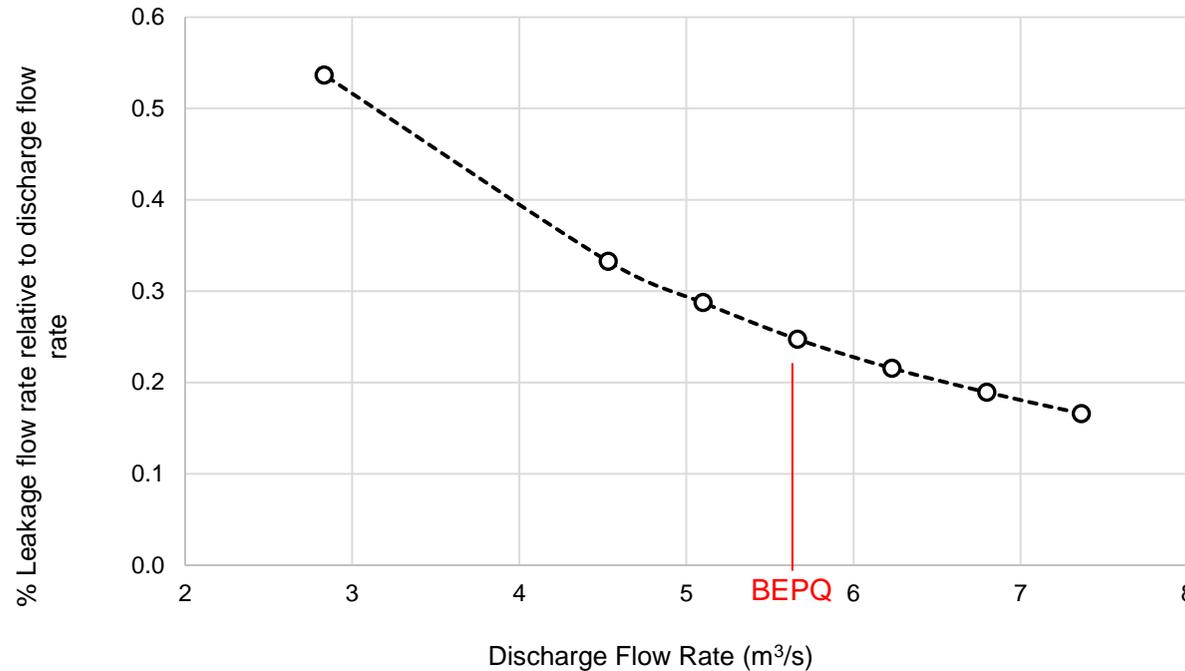
*Figure 10. Leakage flow rate as a % of pump discharge flow rate.*
