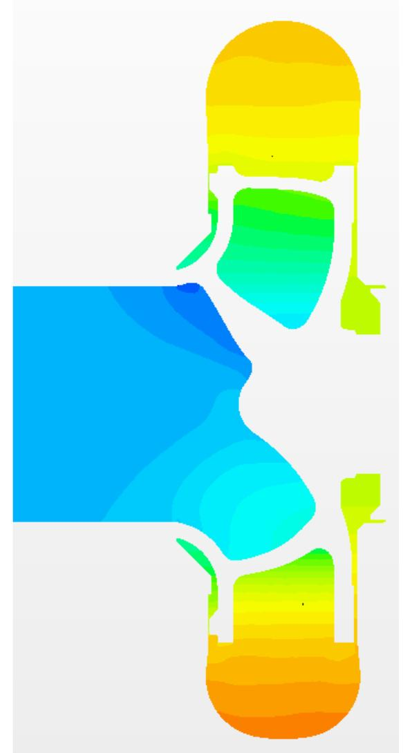
**Figure 11. Static pressure contour plots, on center-planes at 100% BEPQ**
