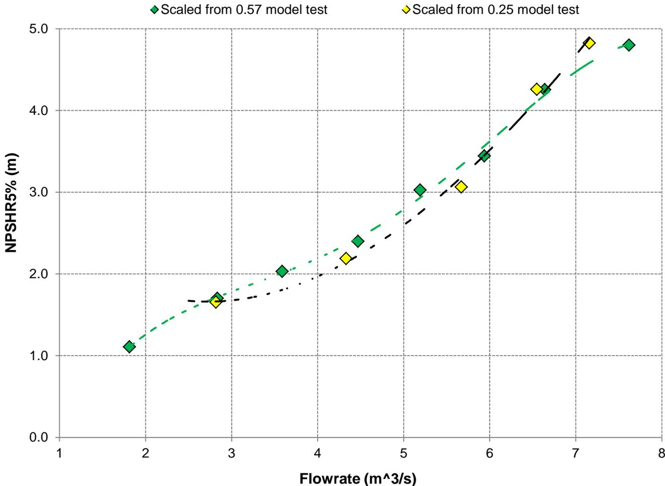
Figure 17 . NPSHR Scaling for the original design.
