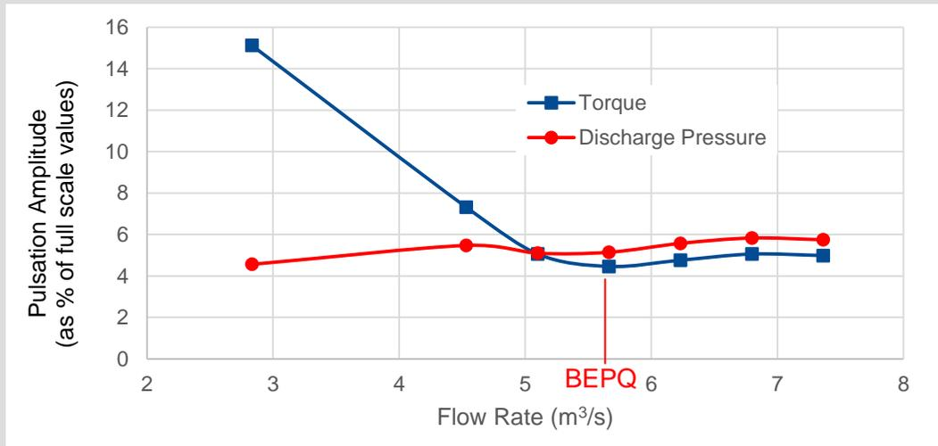
Figure 7. Relative torque and discharge pressure pulsation amplitudes vs. flow rate.
