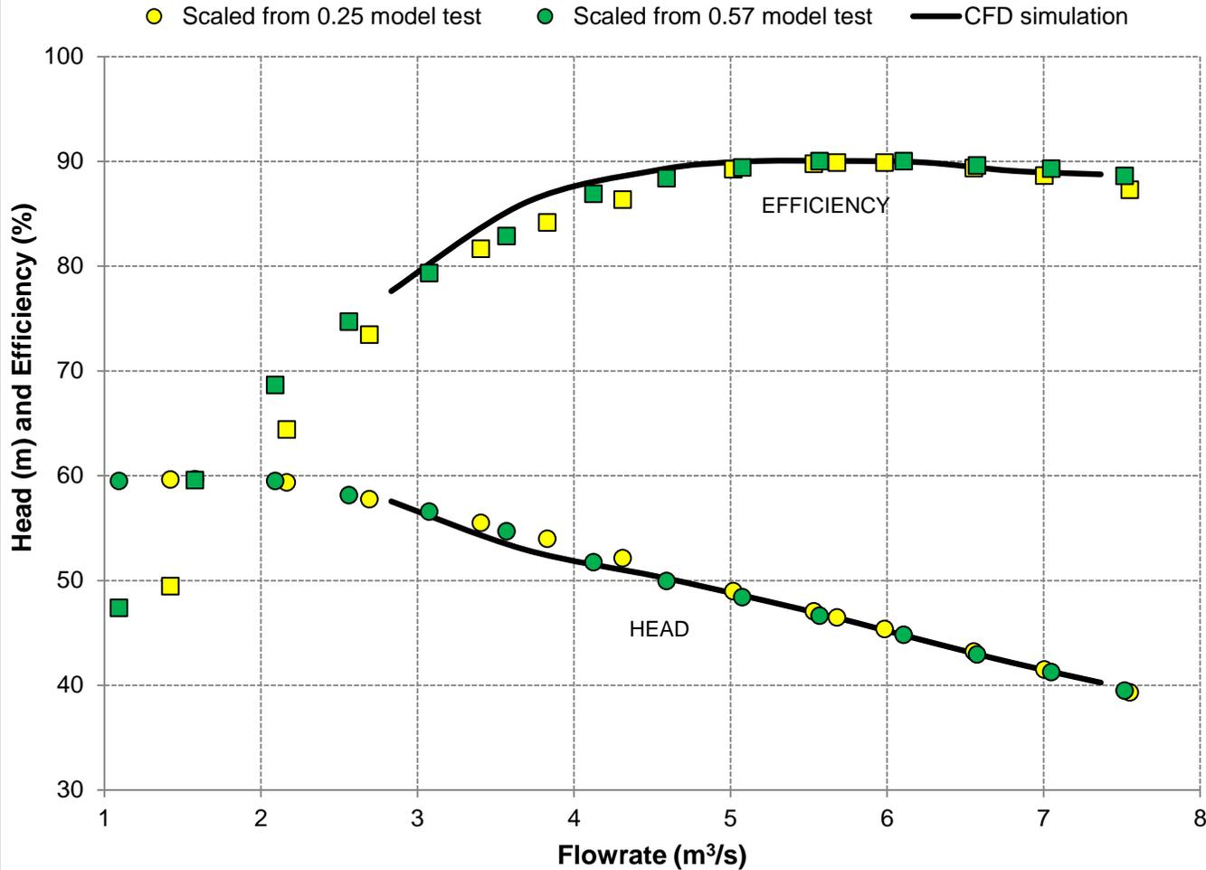
Figure 16. Head and Efficiency scaling for the original design.
