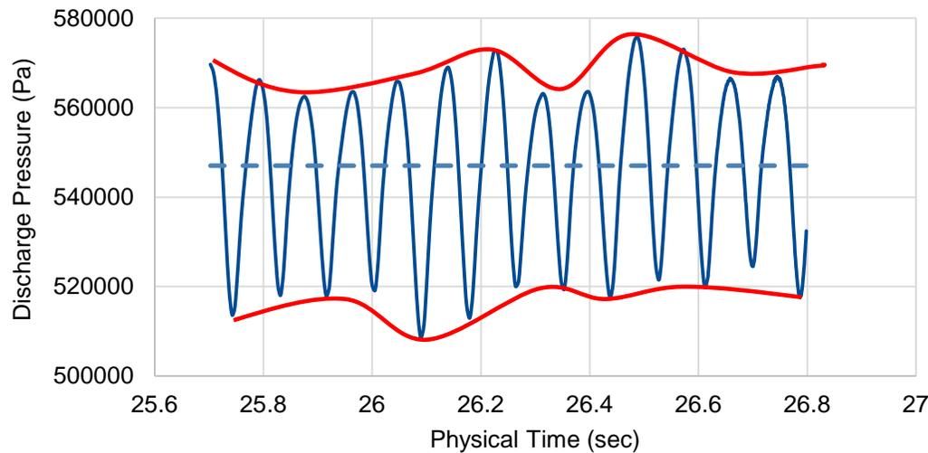
Figure 6. Discharge pressure vs. time @ 45 % BEPQ, dashed line represents mean value.
