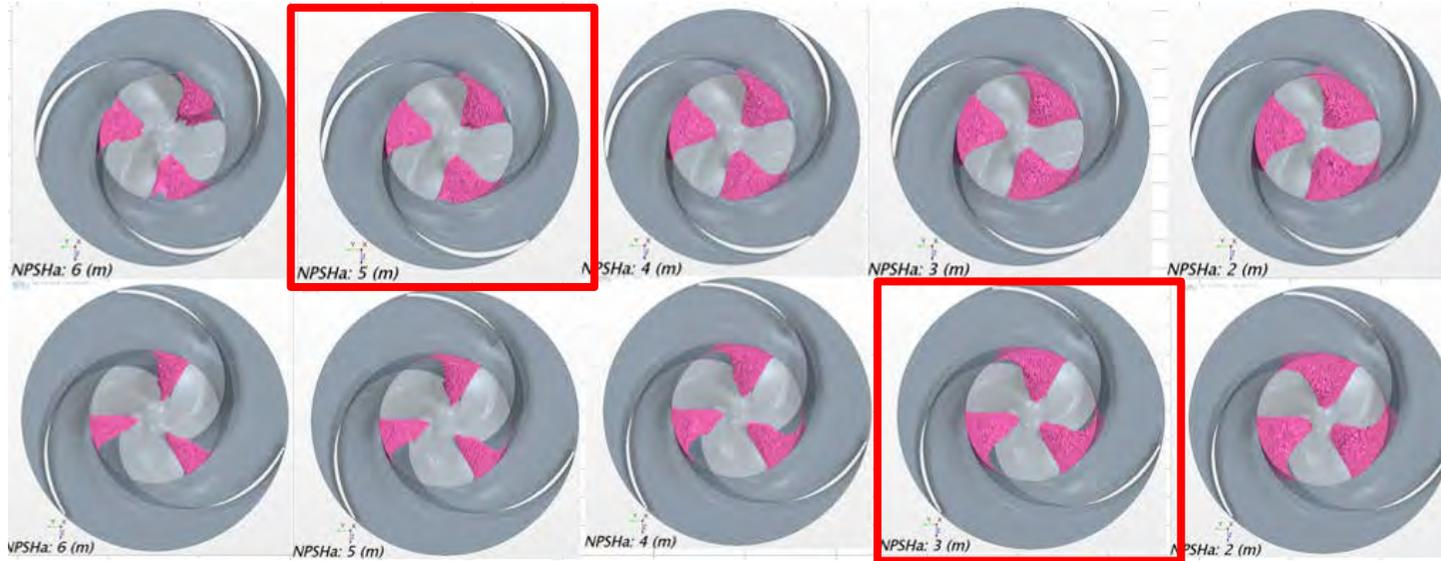
*Figure 18 . Development of “vapor pressure volumes” in two designs.*
