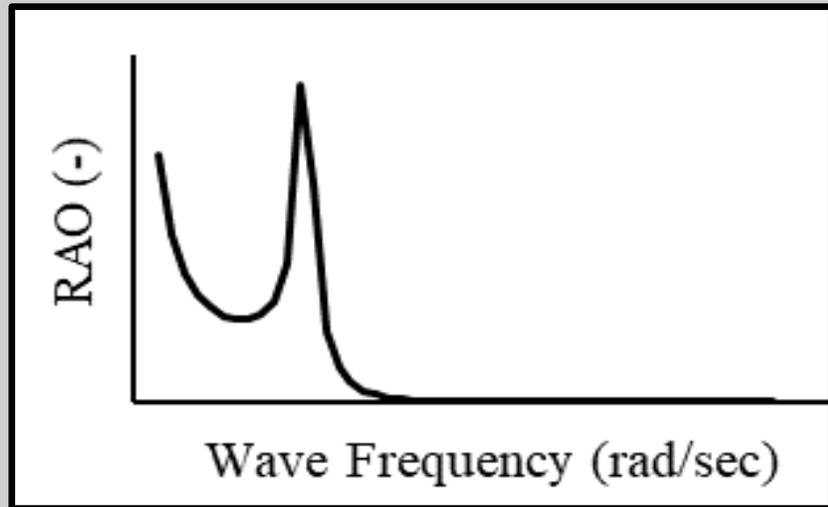
High Wave Frequency: wavelengths too short to induce significant barge motion
