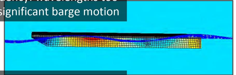
Low Wave Frequency: wavelengths too long to induce significant barge motion
