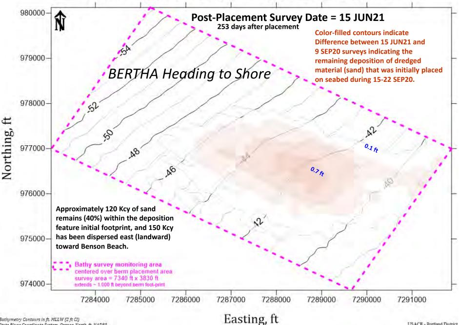
Bathymetry Contours in ft, MLLW (2 ft CI) State Plane Coordinate System, Oregon North, ft, NAD83
