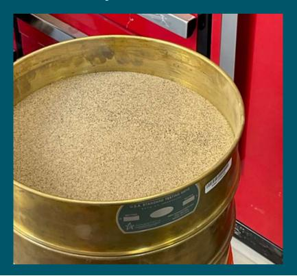
Harford Industrial Minerals, Inc. will combine dredged sediment with other materials into various mix designs, and produce lightweight aggregate for uses such as structural concrete and various fill applications. Final product could serve as local and sustainable alternative to virgin aggregate material generated from quarries.
