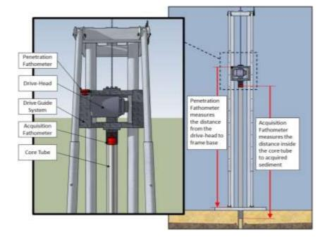
Cores processed utilizing V-SAM produce more accurate estimations for depth of contamination
