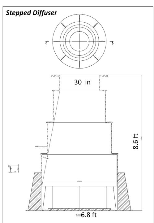
The stepped diffuser allows for <u>simpler fabrication</u> <u>while preserving the rough shape of the smooth</u> <u>diffuser</u>. Concentric cylinders, joined together, form the 'bell' with a flange at the top-most cylinder to attach to the dredging pipe. Eight fins on the bottommost cylinder support a diffuser plate, oriented perpendicular to the flow of incoming slurry to deflect the slurry into a uniform, annular pattern as it leaves the plate.
