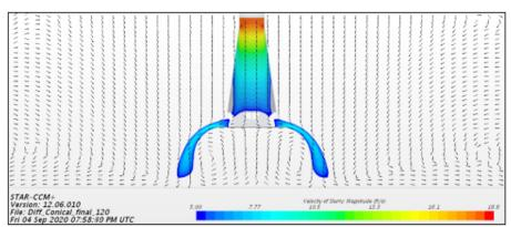
Figure 14: Conical diffuser steady-state slurry velocity profile, 5 ft/s or greater.
