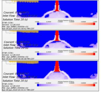
Figure 5: Run 2 at 20 model-seconds showing volume fraction profiles of slurry for original (Top), reduction of one third (Middle), and reduction of one half (Bottom) exit slot heights. Note boundary condition edge effects and how the reduction of one half configuration diffuser is 'full' of slurry.
