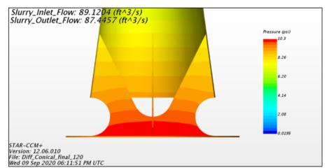
Figure 15: Conical diffuser steady-state stiffener pressures.
