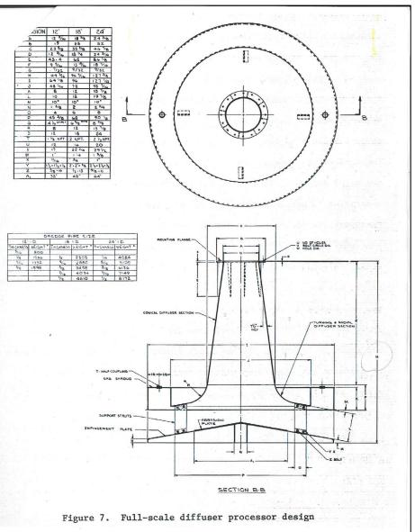
The team determined that these "smooth" designs would be costly to fabricate due to curve expanding geometry----instead the team adopted a "stepped" concept
