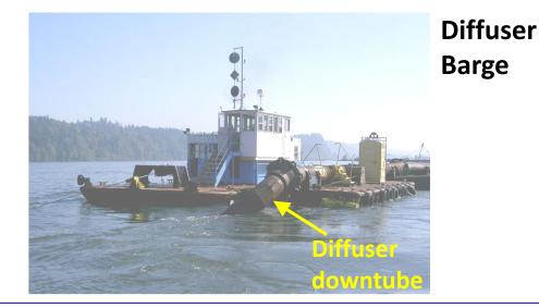
We need a <u>better</u> "tool" to do inwater placement of dredged material within the Columbia River: One that manages energy dissipation, minimizes turbidity, enables shallow water placement (10-20 ft deep), allows controlled deposition of placed dredged material....So that we can build restoration features, or feed the river's sediment budget w/o adverse effect.
