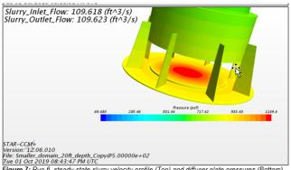
Figure 7: Run 6, steady-state slurry velocity profile (Top) and diffuser plate pressures (Bottom).
