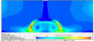
Figure 12: Conical diffuser steady-state turbulent kinetic energy (TKE) profile
