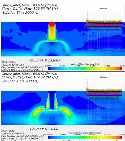
Figure 6: Run 5, steady-state slurry velocity profile (Top) and turbulent kinetic energy profile (Pottom)
