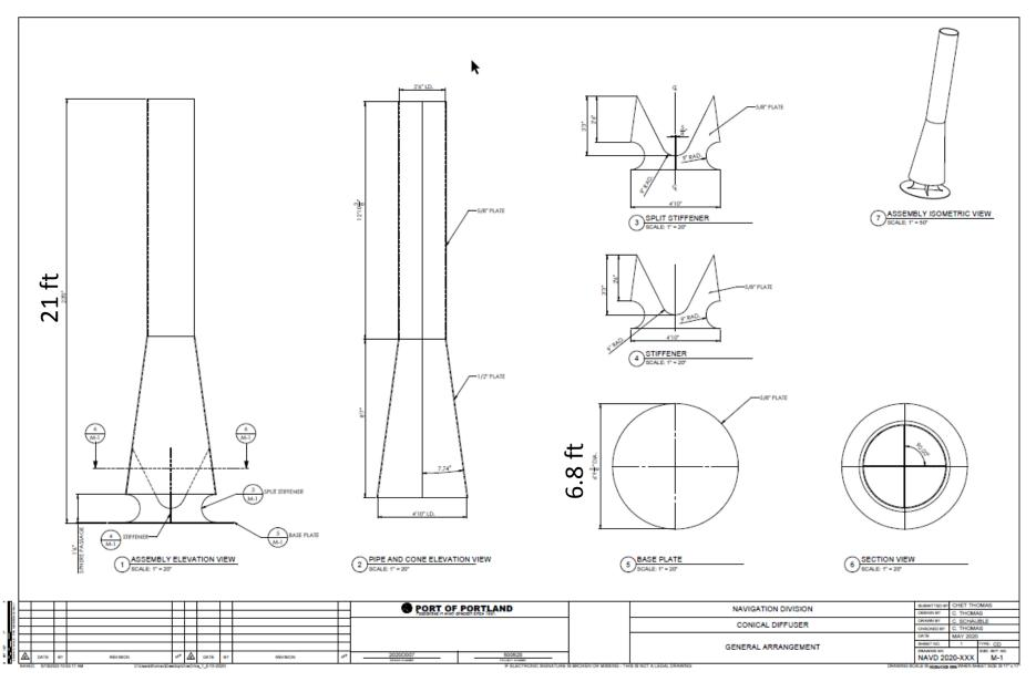
The conical diffuser geometry was defined within CADD and then input into a computational fluid dynamics (CFD) software; Star-CCM+ and modeled numerous times. CADD work was performed by PoP and CFD modeling was performed by Portland District (Aaron Litzenberg and Max Wilson-Fey
