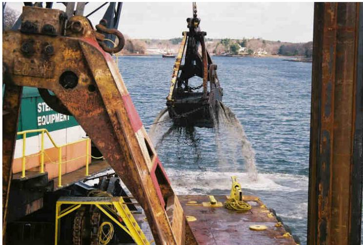
Figure 2: Clamshell dredge in the channel
