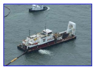
Within a week the first large cutterhead was onsite and mining sand for placement along the northern end of the Chandeleur Island chain on the east side of the Mississippi River.
