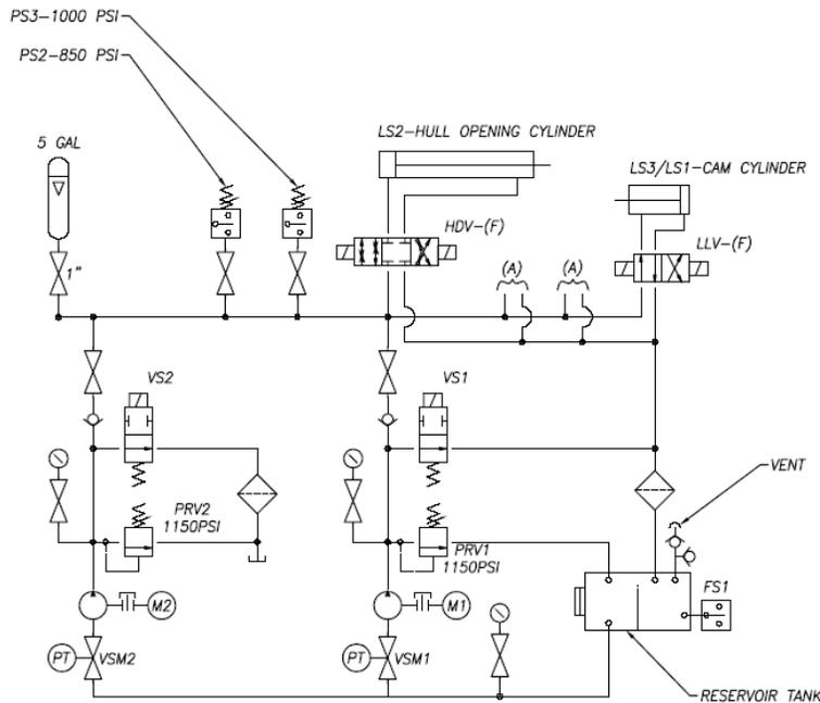
**Simplified Hopper Hydraulic Schematic**
