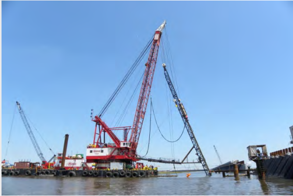
Haakon Maximum Lifting Capacity 400 Tons
