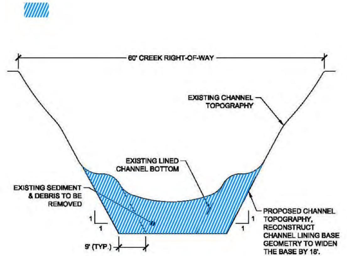
**WIDENING OF CHANNEL BASE - TYPICAL SECTION**
