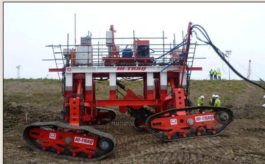
The automated self-levelling system provides a stable, level operational platform.
