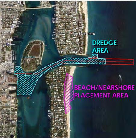
LOCATION: Palm Beach County, Florida DREDGE TYPE: Cutter-Suction/Hopper PLACEMENT: Nearshore QUANTITY: 250,000 CY DEPTH: 37 - 39 feet +2 feet allowable overdepth; settling basins
