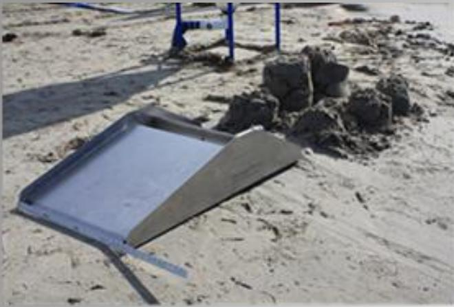
The 2 ft (0.6 m) long Bedload Collector was deployed:
