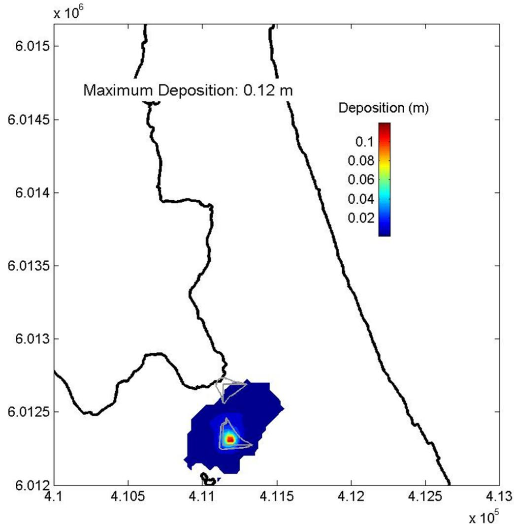
Model derived deposition onto the seabed after 17 days of dredging activity at Berth B1S of the Aurora LNG project
