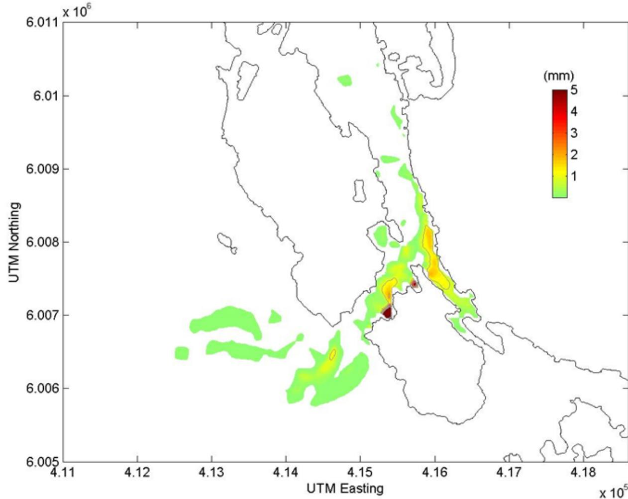
Model derived deposition onto the seabed in Porpoise Channel and the surrounding area after 30 days of dredging activity in January.
