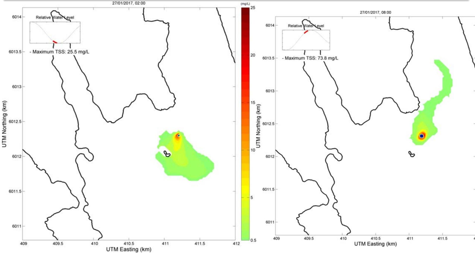
Model derived maximum SSC values in the water column on January 27 following an ebb tide (left panel) and following a flood tide (right panel)
