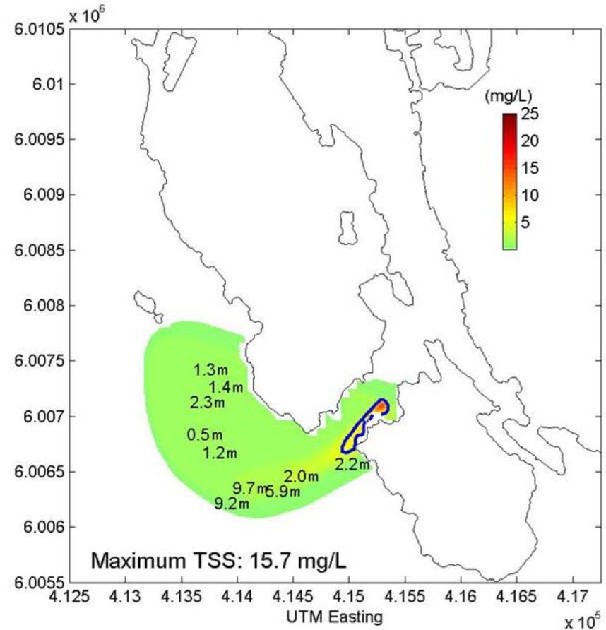
Model-derived SSC (mg/L above background, maximum value in the water column) at ebb flow (left panel, 21:00 January 12) and at flood flow (right panel, 21:00 January 12).
