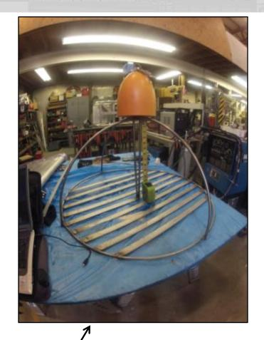
Prototype deployable deposition meter, via Curtis Roegner-NOAA. These are designed to go "over the side" and be retrieved like crab traps.
