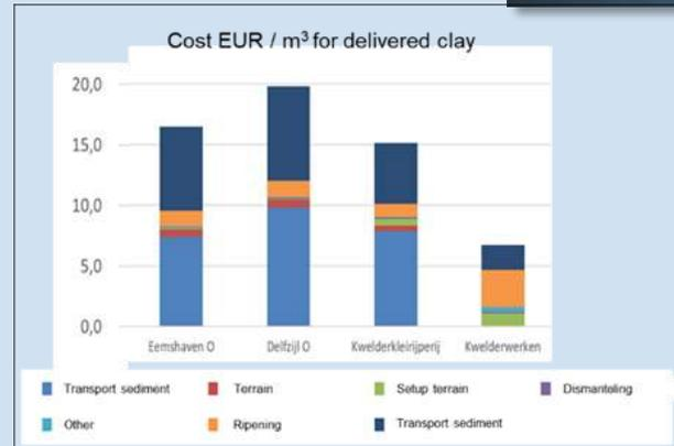
Above: Aerial photo of the dewatering basin after deposition of fresh dredge sediments. Left: Results of the cost analysis for producing clay from ripening dredge sediments for sediment from the ports of Eemshaven, Delfzijl and from salt marshes distant from the clay.
