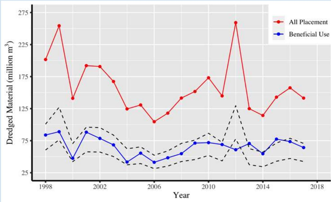
Dredging placement for USACE navigation dredging from 1998–2017. Dashed lines represent 50% and 30% thresholds of all dredged material placed and are shown to demonstrate what percentage beneficial use is of all placement (Adapted from Searcy Bell et al. 2021).
