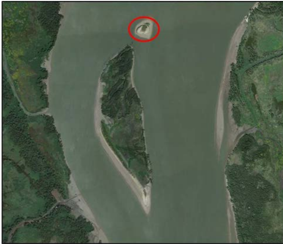
Figure 1: Horseshoe Bend Island, a 35 ha island supported by strategic dredge material placement. Note the small dredged material mound (circled) placed immediately upriver (north) of the island. Image dated October 28, 2012 (imagery provided by USACE MVN).
