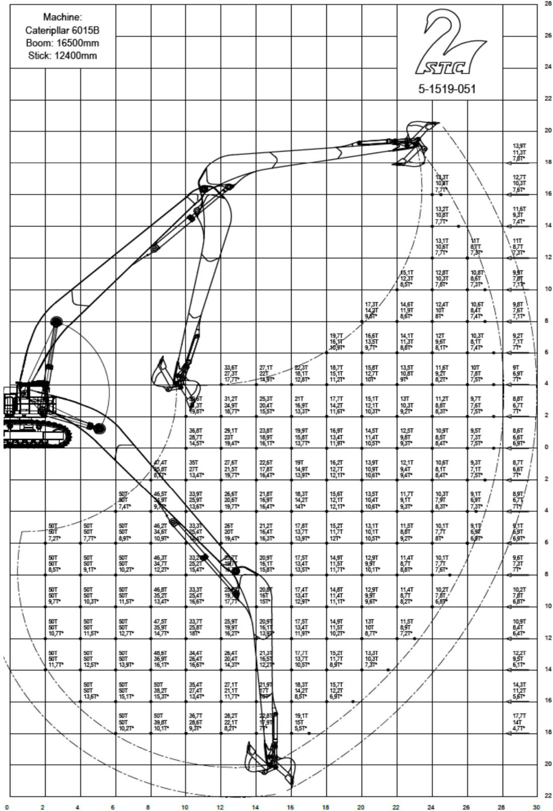
Figure 3. Final working range and lifting capability of customized long-reach excavator.
