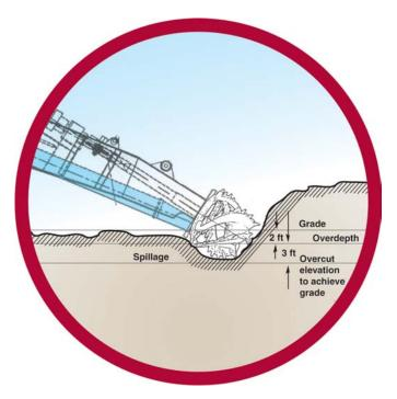
Figure 7 - Typical cutting below grade level
