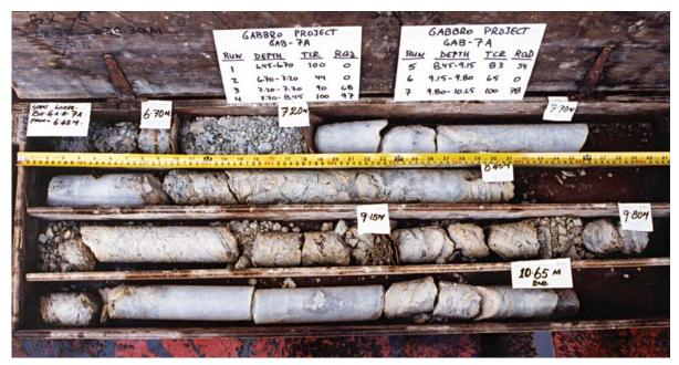
Figure 9 - Rock core photo log
