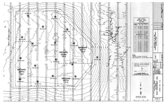
Figure 6 - Good boring coverage in borrow area
