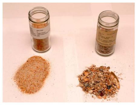
Figure 13 - Sand samples described as Sand with "some shell" (left) and with "shell hash" (right)
