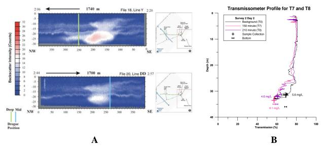
Figure 7. Profile plots of ADCP data collected along Lines Y and DD (Plume 2) displaying residual acoustic backscatter intensity within the water column to illustrate plume morphology 126 to 177 minutes after the dredged material disposal event at Point B (A). Profile plot of percent light transmission and sensor depth acquired during CTD sample intervals T7 and T8 for Plume 2 (B).
