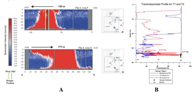
Figure 4. Profile plots of ADCP data collected along Lines F and G (Plume 3) displaying residual acoustic backscatter intensity within the water column to illustrate plume morphology 2 to 10 minutes after the dredged material disposal event at Point B (A). Profile plot of percent light transmission versus sensor depth acquired during CTD sample intervals T1 and T2 during Plume 3 (B).
