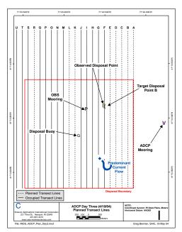
Figure 2. Basemap displaying a subset of the predetermined ADCP survey lanes established over RISDS.
