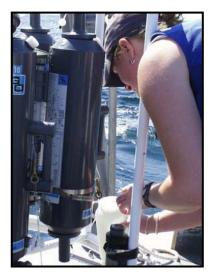
Figure 3. Images of the Seabird SBE32 Carousel unit employed as part of the plume monitoring surveys performed at RISDS.
