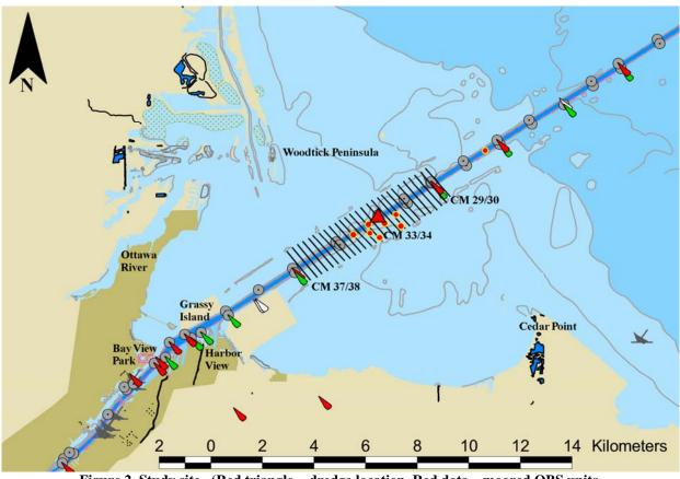
Figure 2. Study site. (Red triangle = dredge location, Red dots = moored OBS units, Parallel black lines = ADCP transects. See text.)
