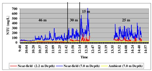
Figure 4. Near-field turbidities at various depths and distances from the bucket.
