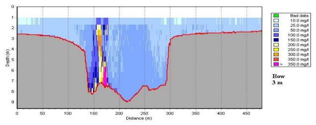
Figure 8. Vertical profile of TSS concentrations at 3 m from the source (Survey TCSB).
