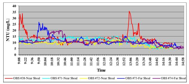
Figure 6. Turbidities recorded at 5 stations over shoals adjacent to the navigation channel.
