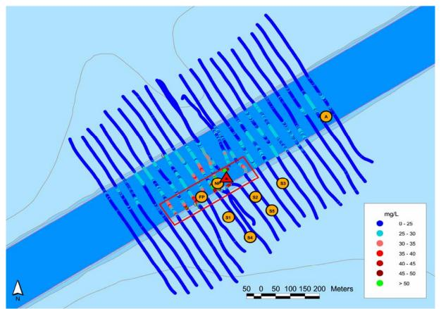
Figure 7. Depth-averaged suspended sediment concentrations during bucket dredging operations in the Maumee Bay navigation channel. Dredge location indicated by red triangle. Orange circles are OBS stations.
