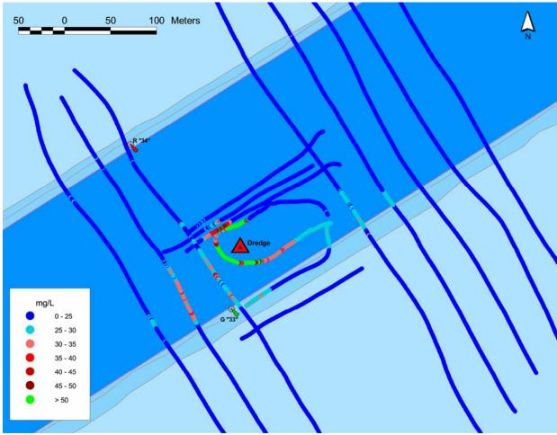
Figure 13. Depth-averaged suspended sediment concentrations during dredging operations in the Maumee Bay navigation channel. Red triangle indicates position of dredge.
