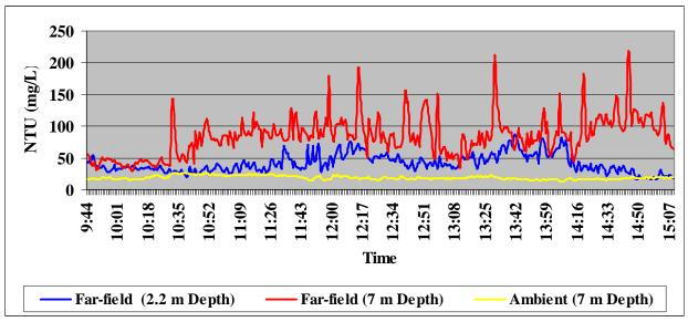
Figure 5. Far-field turbidities at 2.3 and 7.5 m water depths at a distance of 95 m from the bucket. (Note: Ambient sensor deployed at 2.2 m failed.)
