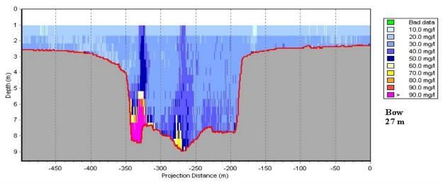
Figure 9. Vertical profile of TSS concentrations at 27 m from the source (Survey TCSB).
