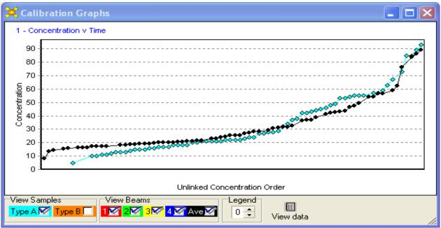
Figure 3. Comparison of gravimetric and acoustic estimates of TSS concentration for all samples in rank order. Gravimetric measurements are represented in blue, whereas acoustic estimates are in black.
