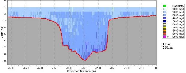
Figure 12. Vertical profile of TSS concentrations at 201 m from the source (Survey TCSB).
