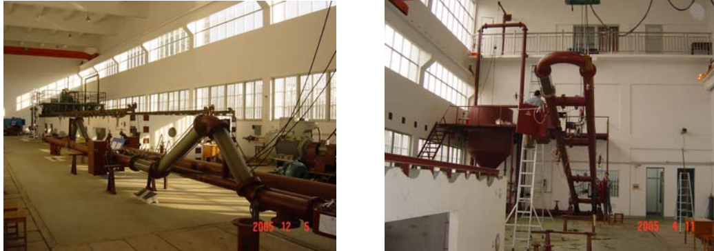
Figure 1. 315kW-DN200 pump-pipeline slurry transport stand at Hohai University, China.
