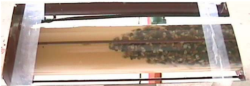
Figure 3. Observation of the mixture flow with a mirror underneath the transparent plexi-glass pipe.
