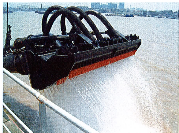
Figure 6. Jetting as applied on dragheads. Left: Jetting from the heel of an IHC Mudhead (1980) Right: Jetting in the Wild Dragon through heel and teeth bars (2004)
