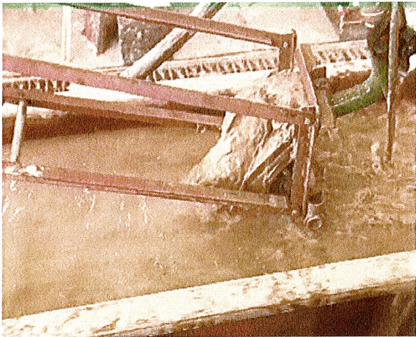
Figure 15. The very fine sand from the bank in the Yangtse. Left: Testing the material characteristics during a test cut. Right: The sieve curve documents the very fine characteristics.
