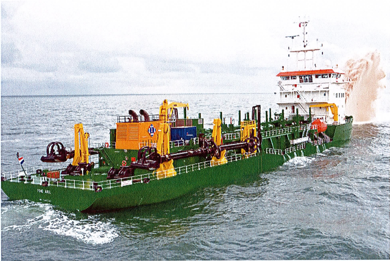
Figure 18. TSHD ABUL, fitted with two WILD DRAGONS (Californian drag-heads on deck) being tested near Goeree in the North Sea, near The Netherlands coast.
