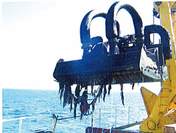
Figure 20. The Abul WILD DRAGON drag-head having caught burlap bags. In the meantime, WILD DRAGONS have been delivered elsewhere and applied in production jobs.
