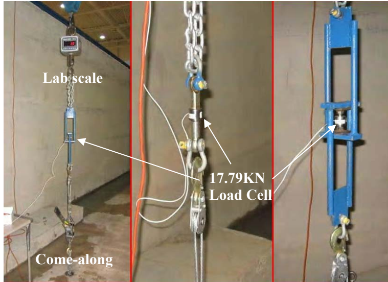
Figure 3. Calibration procedure for the calibrator cell
